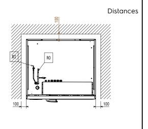
**Electric** Circuit breaker required Supply voltage: 380-415 V/3N ph/50/60 Hz Heating power: 6.4 kW Water: Drain line size: Pressure, bar min: 0 Installation: Clearance: 5 cm on sides and back. Capacity: 150 kg Max load capacity: Number and type of grids: 20 (GN 2/1; 600x400) Number and type of basins: 30 (360x250x80h) **Key Information:**
